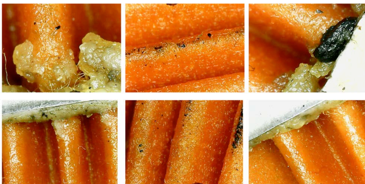
Figure 6. Visual impression of clogged filter contacted to B100 for 3500 hours
