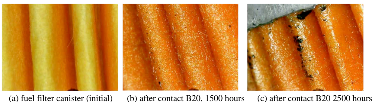
Figure 5. Visual impression of clogged filter for engine fuelled B20
